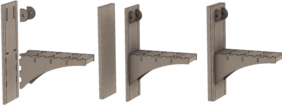
Assembly scheme the students would follow to attach their structures to the plywood back plate
